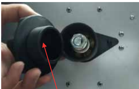
(1) Remove the spool retaining nut.
